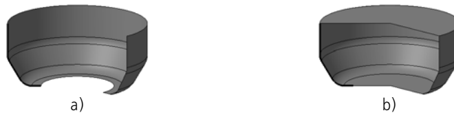
Fig. 2.6.7. Spheroid and toroid construction (section—sketch—marked with a thickened line): a) spheroid, b) toroid
