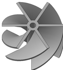
Fig. 2.7.23. Example of array along circular grid
