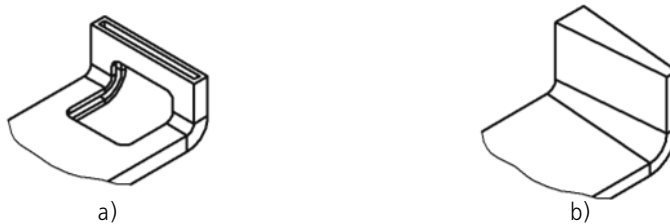
Fig. 2.4.91. Examples of operations that make impossible unbending of the bend: a) casing, b) slope
