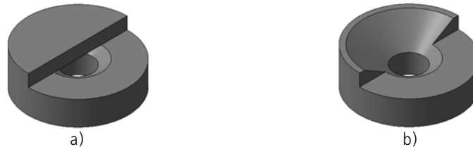
Fig. 2.3.55. Creation of a hole with countersink: a) the Process canopy option is disabled; a) the Process canopy option is enabled
