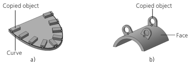
Fig. 2.7.37. Example of array instances positioning: a) with orientation by curve; b) with orientation by surface
