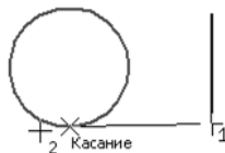
Fig. 3.2.63. Example of constructing a subsequent line segment
