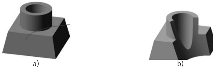
Fig. 2.3.51. Cutting a part component by sketch: a) initial state of the part, the sketch of the surface to be cut off is shown, b) result of cutting operation
