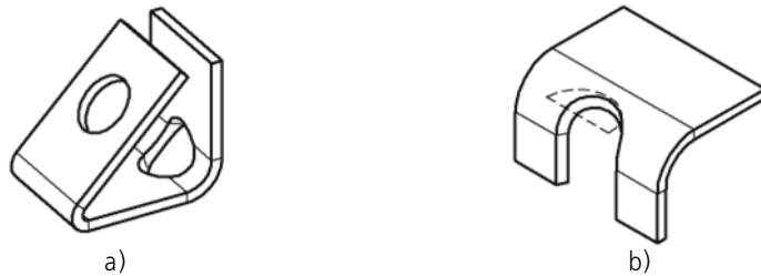
Fig. 2.4.92. Example of holes and cuts that make impossible unbending of the bend
