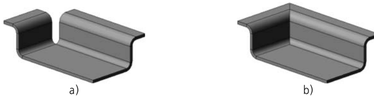
Fig. 2.4.70. Bend along a chain of edges: a) with no corner capping, b) with capping (one of the options available)
