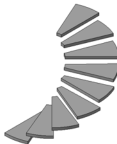
Fig. 2.7.26. An example of an array along circular grid with instances' offset along the axis
