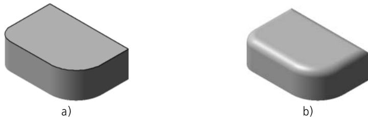
Fig. 2.3.42. Fillet: a) to construct fillet, the upper face is shown, option is enabled; b) result of fillet construction
