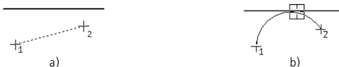
Fig. 3.2.65. Constructing the first arc of a line tangent to an object: a) selecting the start and end point, b) selecting the object
