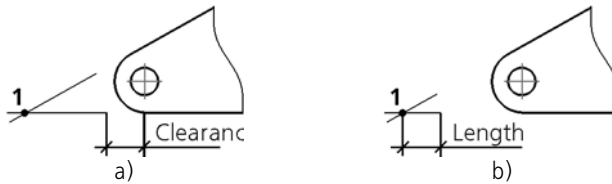
Fig. 3.3.99. Drawing extension lines when setting a non-zero value: a) gap; b) length
