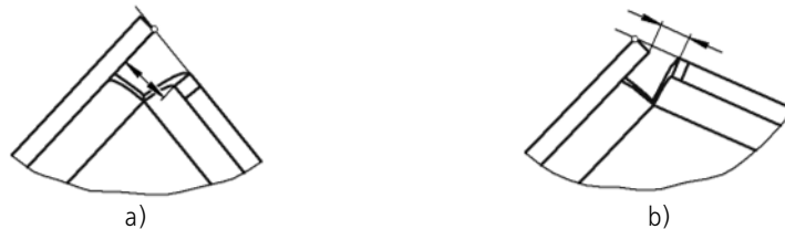
Fig. 2.4.62. In capping with overlap: a) closable acute angle, b) closable obtuse angle
