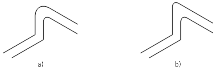
Fig. 2.5.53. Rounding segments of an equidistant curve: a) without saving radii; b) with saving radii
