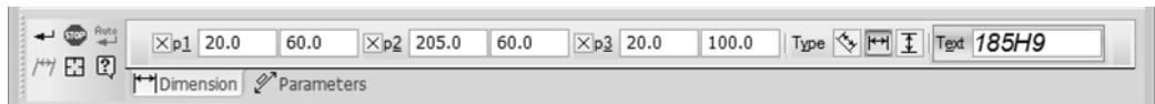
Fig. 3.3.2. Usage of the Dimension tab of the Property bar while specifying a linear dimension
