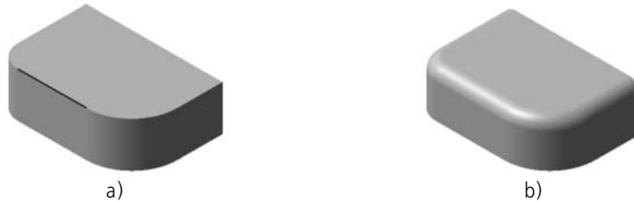
Fig. 2.3.43. Fillet: a) to construct fillet, one edge is shown and Continue by Tangent option is enabled; b) result of fillet construction
