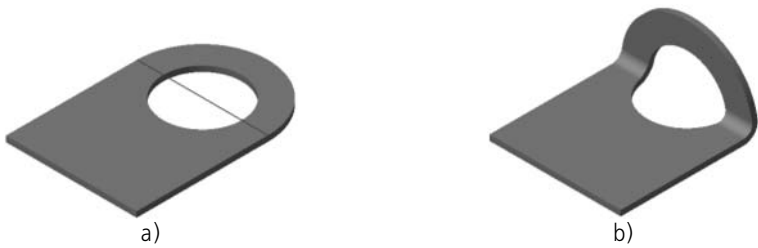
Fig. 2.4.43. Bending a part with a hole: a) position of the bend line, b) the result of building
