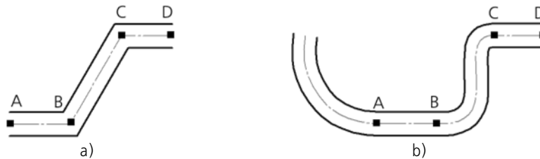
Fig. 3.2.77. Adding segments to the multiline: a) initial multiline; b) result of addition
