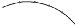
Fig. 3.2.8. Example of three points drawn along an arc at a distance of 5 mm from the reference point
