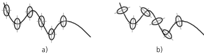
Fig. 3.4.13. Copying an ellipse along a spline: a) without additional rotation of the copies to the normal, b) with additional rotation of the copies to the normal
