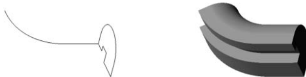
Fig. 2.3.30. Section, guide and swept feature
