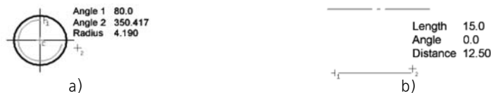
Fig. 1.4.8. Displaying object parameters next to the cursor: a) when creating an arc using three points, b) when creating a line parallel to an existing line
