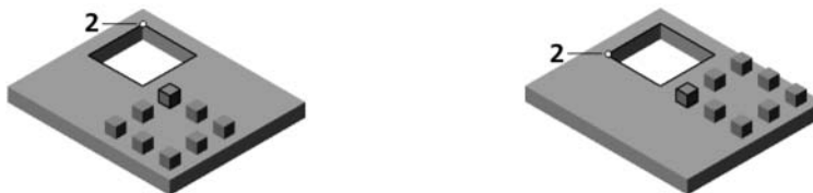
Fig. 2.7.31. Relation between disposition of copies and location of the start point of the curve. (copying path and the object to be copied are highlighted, starting point is indicated by a circle)
