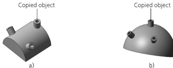
Fig. 2.7.45. Example of orienting array's instances in radial direction: a) positions are set in cylindrical coordinates; b) positions are set in spherical coordinates.
