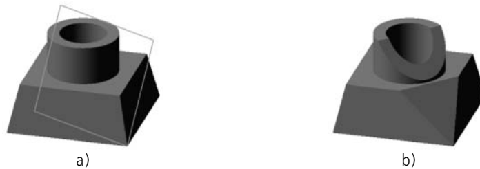
Fig. 2.3.50. Cutting a component of the part by plane: a) initial state of the part (cutting plane is denoted relatively), b) result of cutting operation
