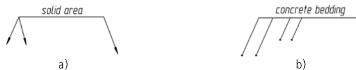
Fig. 3.3.55. Leader Length: Leader branches a) from the start and the end of the shelf, b) parallel
