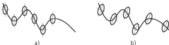
Fig. 3.4.10. Copying objects: a) maintaining the rotation angle and the scale, b) by changing the rotation angle and the scale
