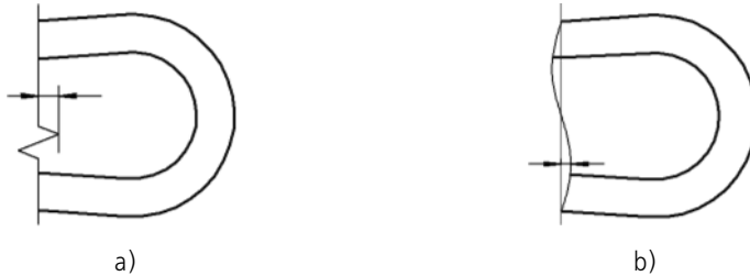
Fig. 3.5.18. Height: a) of a bent line, b) of a wavy line (the middle line is also shown in the figure)
