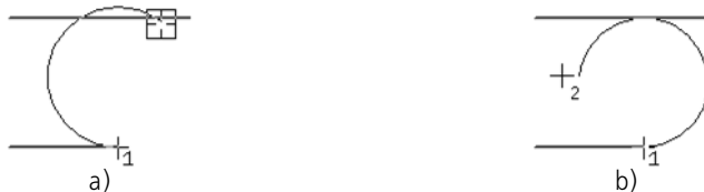
Fig. 3.2.67. Constructing a subsequent arc of a line tangent to the previous segment and to an arbitrary object: a) object selection, b) specifying the arc endpoint
