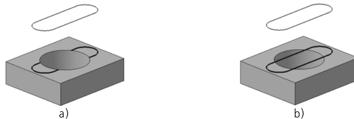
Fig. 2.5.60. Result of the sketch line projection on a face with a hole: a) the Trim by borders option is on; b) the Trim by borders option is off
