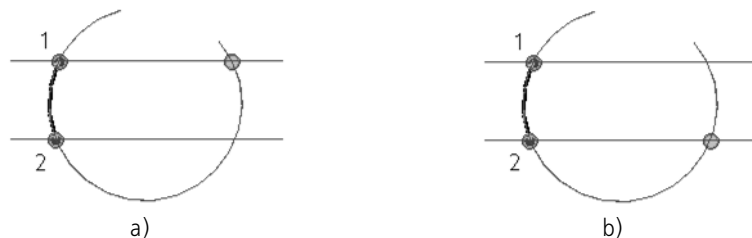
Fig. 2.5.50. Ghost of curve trimmed by two objects: a) without pressing the <Ctrl> button; b) with pressing the <Ctrl> button
