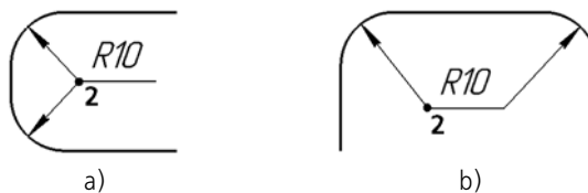
Fig. 3.3.27. Radial dimension of the shelf with two branches a) From Shelf Start, b) From Shelf End.
