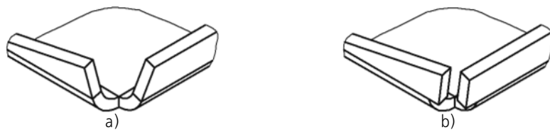
Fig. 2.4.56. Butt capping: a) original part status, b) the result of capping of angle (the gap is not equal to zero)
