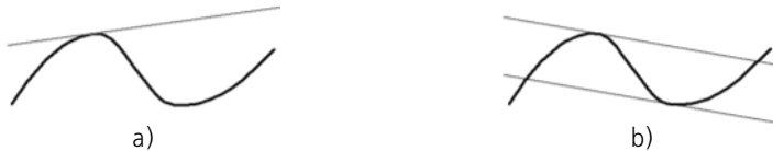
Fig. 3.2.14. Line tangent to the spline: a) passing through a spline point, b) having a specified tilt angle
