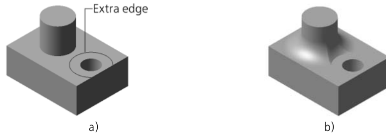
Fig. 2.6.32. Using an edge resulting from face's splitting: a) initial state of a part, b) result of a rounding by maintaining "cliff" edges
