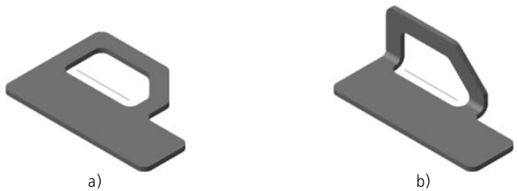
Fig. 2.4.44. Using an auxiliary axis as the bend line: a) location of the axis, b) the result of building
