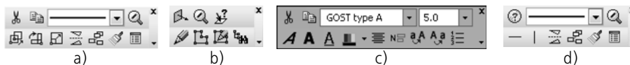
Fig. 1.2.10. The context toolbar when you select: a) a geometric object in a drawing or fragment, b) a body face in an assembly, c) a text fragment in a text document, d) a geometric object in a 3D element sketch
