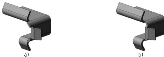
Fig. 2.4.75. Bend along a chain of edges connected by bends: a) without angle release, b) with angle release
