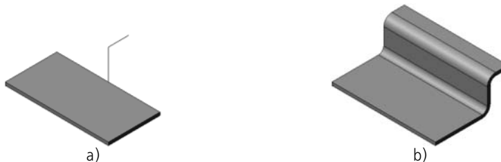
Fig. 2.4.66. Bend By Edge : a) initial state of the model and the bend sketch, b) construction result
