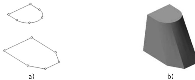
Fig. 2.3.37. The arc in the upper section is divided into three mating parts.
