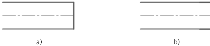
Fig. 3.2.80. Straight-line limiter: a) with zero height; б) with the height greater than zero
