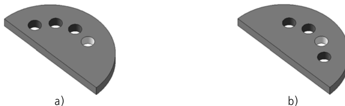
Fig. 2.7.28. Changing instances' position in an array against the base instance (the base instance is highlighted in white color): a) base instance with number (1.1); b) base instance with number (1.2)
