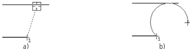
Fig. 3.2.68. Constructing a subsequent line arc tangent to an arbitrary object: a) object selection, b) specifying the arc endpoint
