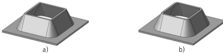
Fig. 2.4.100. A drawn cutout with a slope on side walls and a round on side edges: a) the rounding radius is equal zero, b) the rounding radius is greater than zero
