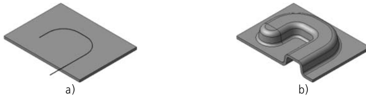
Fig. 2.4.104. The beat exceeding the limits of the basic face: a) the beat sketch; b) the result of building
