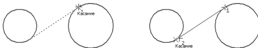
Fig. 3.2.59. Example of constructing the first line segment
