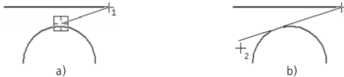
Fig. 3.2.62. Constructing a subsequent line segment tangent to another object: a) selecting the object, b) selecting the segment endpoint
