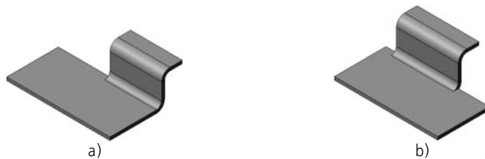
Fig. 2.4.67. By length Bend: a) in one direction from the sketch plane, b) in both directions
