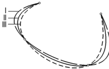
Fig. 3.2.52. Splines with different methods of forming point parameters: I – Linear , II – Centripetal , III – Chord length
