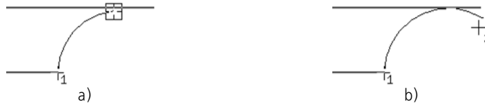
Fig. 3.2.70. Arc by a normal, tangent to an object: a) object selection, b) specifying the arc endpoint
